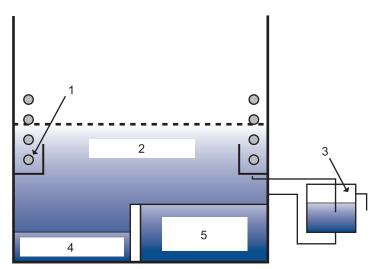
Key 1: condensate trough 2: vapour zone 3: water separator
